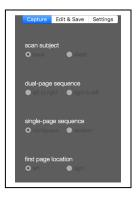
Once the main window opens, the session configuration can still be changed before any scan is made using the radio-button controls at the top of the 'Capture' page. After a capture is made, it is no longer possible to change the session configuration.
